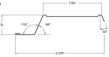
RC Super meets the resilient channel requirements of the following UL assemblies: L521, L546, L547, L550, L558, L562, L563, L569, L570, L574, L576, L579, L589, L590, L592, L593, L598, M501, M502, M503, M506, P515, P522, P524, P531, P533, P535, P538, P541, P545, P549, P551, P552.
